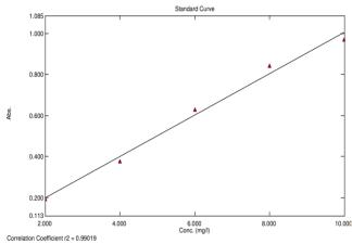
**Result:** The Calibration curve of Sumatriptan Succinate plotted at 227nm and correlation coefficient  $(R^2)$  of determination was 0.99.
